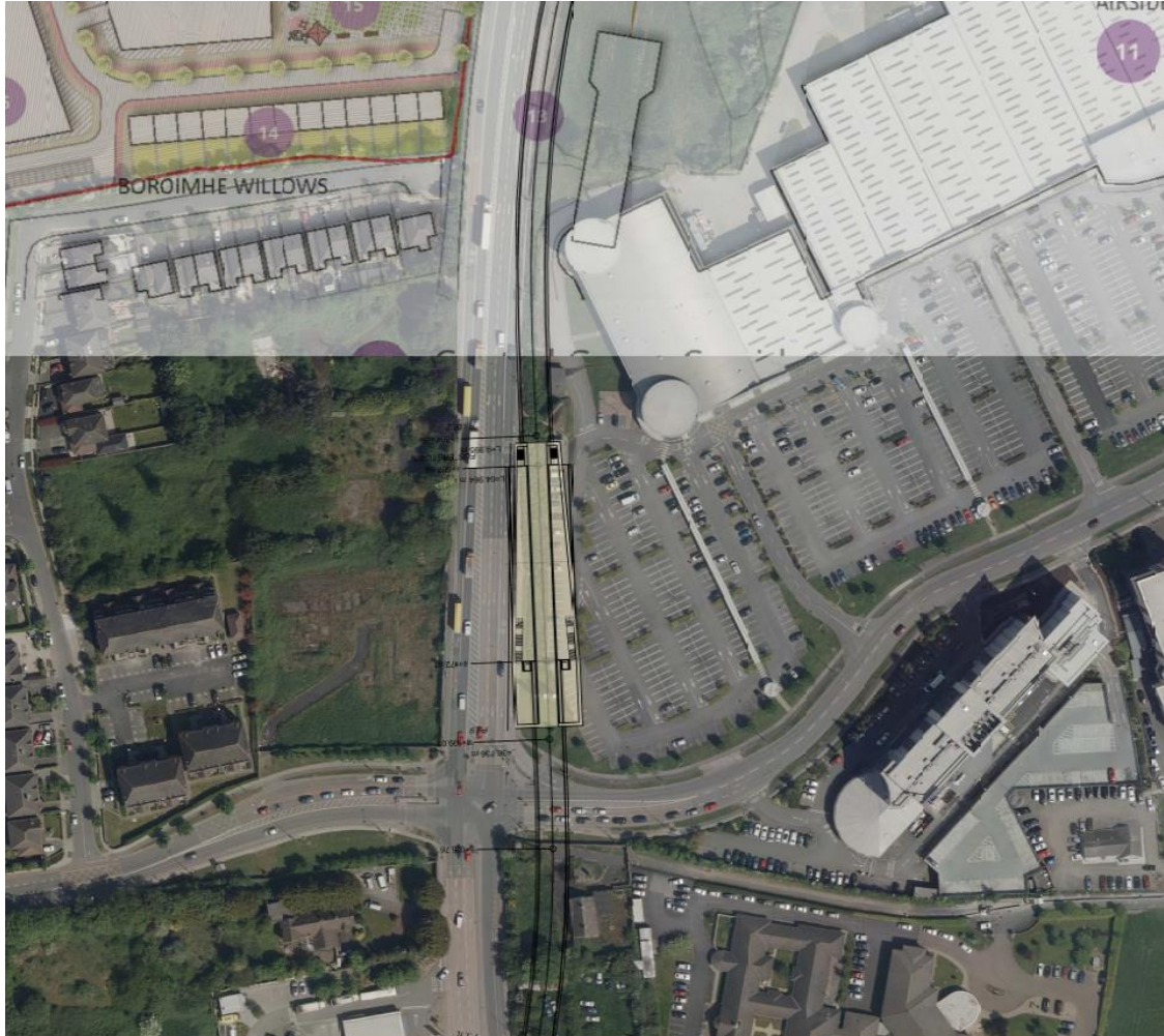
Figure 3.10 Alternative Option 2B: alignment moved west to avoid Airside Building and station moved south
