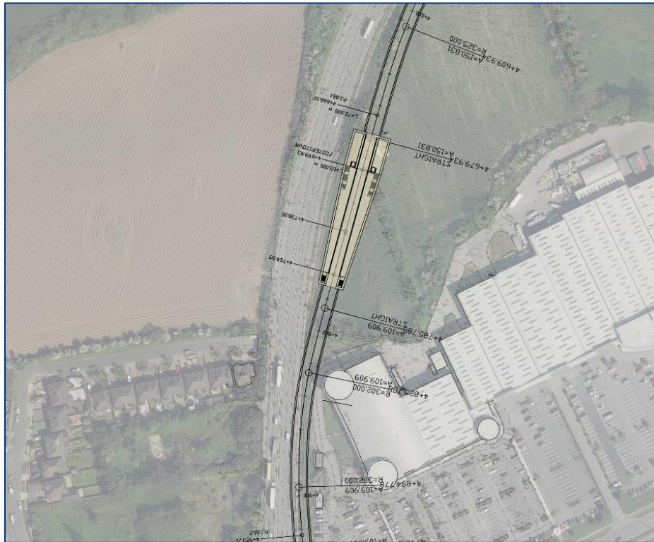
Figure 3.6 Alternative Option 2A: alignment moved west to avoid Airside Building and station moved north
