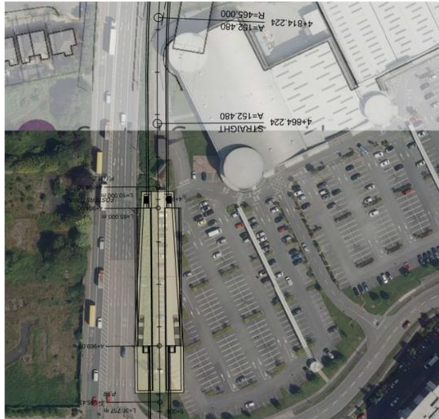
Figure 3.5 Alternative Option 1B: Minor displacement of the alignment and Station moved to the South
